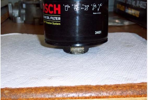
The filter weighs 13 ounces when new. The filter in the picture weighs 23 ounces.
