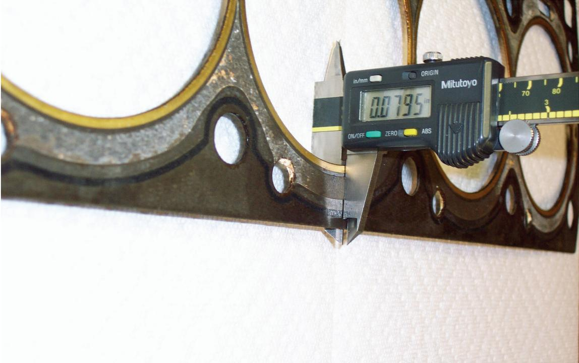
A gasket exposed to coolant with organic corrosion inhibitor swells much more. This gasket was used with Dex-Cool for one year.
