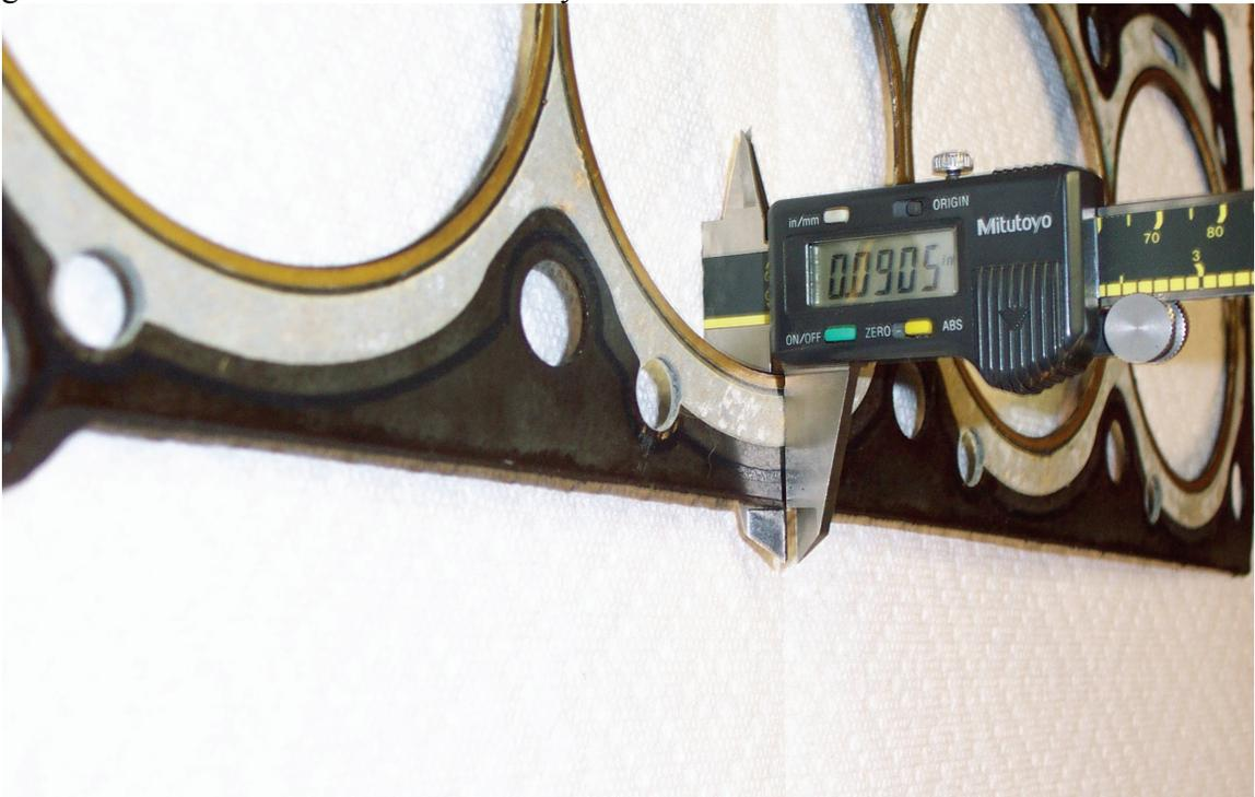
I believe that this is evidence that the fiber material is softened by coolant with an organic corrosion inhibitor. If the fiber is softened, it is possible that the sealing ring around the cylinder can loosen because it is crimped over the fiber.
