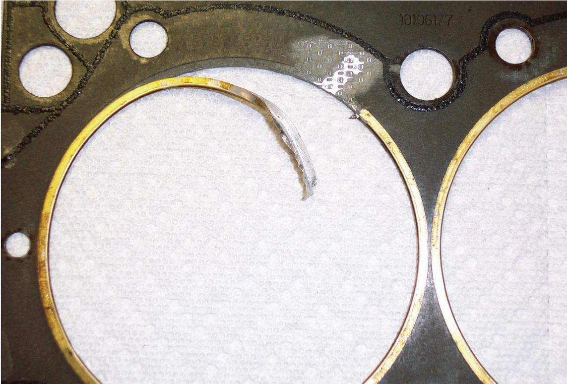
If the fiber softens the support for the sealing ring will lessen, and the ring can compress and fit looser between the cylinder liner and the cylinder head.
