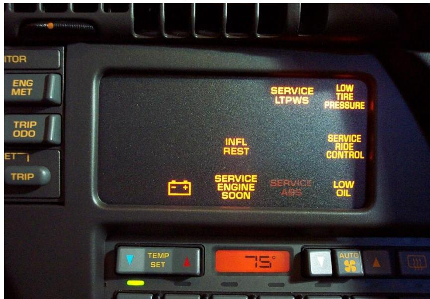
This display is for a '91 car. '90 cars are the same except there is no Low Oil indicator on a '90. These lamps should go on for about three seconds. Some will go out after three seconds. They should all go out when the engine is started. Lamps that don't go on suggest malfunctions or tampering. Lamps that remain on when they should not, are indications of a malfunction.
